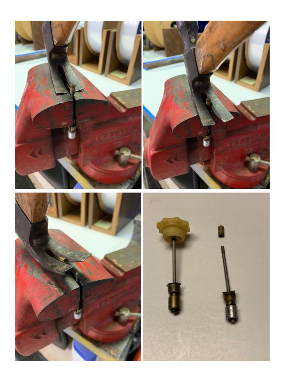
4. Now place your new Cap on a solid flat surface, and simply tap the Rod Assembly into the new Cap until it seats. (Completed assembly shown below is not fully seated--the splines will end up completely (or 95%) inside the brass cap).
