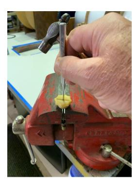
3. Now tighten the Rod Assembly in the vice as shown in the photo. Use a lever and gently pry <u>straight up</u> (not and an angle!) to remove the pressed-on brass fitting from the splined rod as shown in the following photos.
