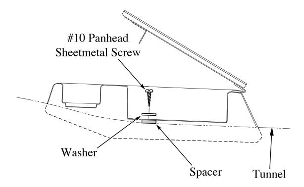
The recommended fastening method is to screw through the storage compartment and into the tunnel (see sketch). This is how consoles were installed at the factory.
