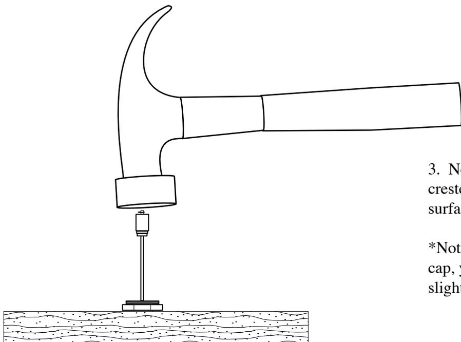
3. Now simply tap the rod into the new MG crested cap with a hammer\*. Use a firm, flat surface, and let the rod guide itself home.
