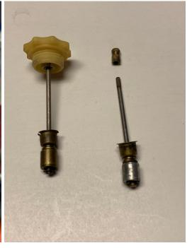
4. Now place your new Cap on a solid flat surface, and simply tap the Rod Assembly into the new Cap until it seats. (Completed assembly shown below is not fully seated--the splines will end up completely (or 95%) inside the brass cap).
