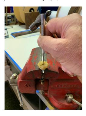
3. Now tighten the Rod Assembly in the vice as shown in the photo. Use a lever and gently pry <u>straight</u> <u>up</u> (not and an angle!) to remove the pressed-on brass fitting from the splined rod as shown in the following photos.
