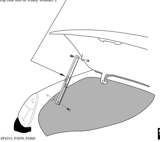
Hood Prop may be located on either side of the engine compartment, depending on model year. Installation is the same on either side.
