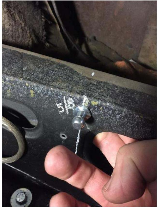
3. Close your access panel, and measure to the top bracket location as shown. Start by drawing a line parallel to the edge of the panel, off-set by 2.5 inches.
