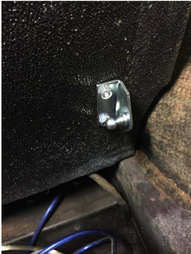
7. Snap on the Strut, then close and open the access panel to ensure everything operates smoothly. If you need to remove the Strut, simply put a small flat blade screwdriver under the black locking spring at the end of the Strut, and pull the Strut free.
