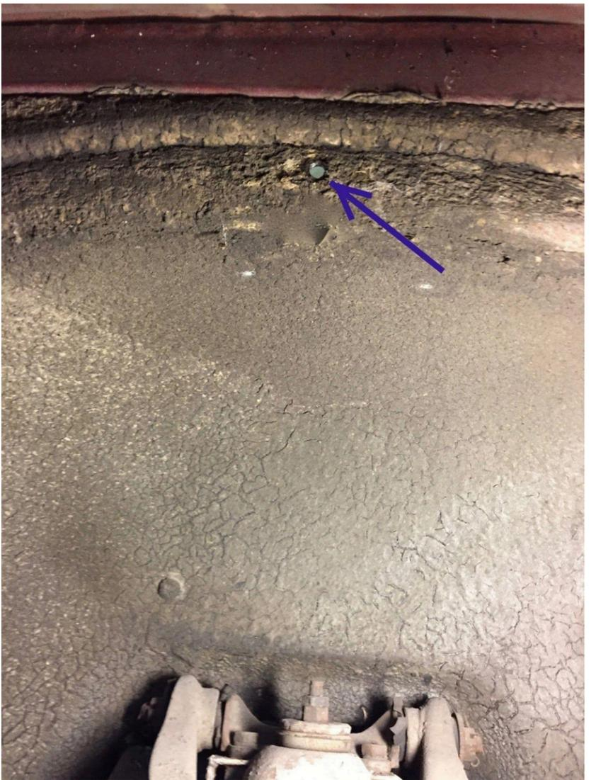
6. Now install the ball stud, using a flat washer and nut on the back side. Hold the front side still with a wrench as shown. Use a drop of thread lock on the nut to make sure it can't vibrate loose.. Note: if you have a thick layer of undercoating, you may have to remove some of it to get the nut fully onto the stud.
