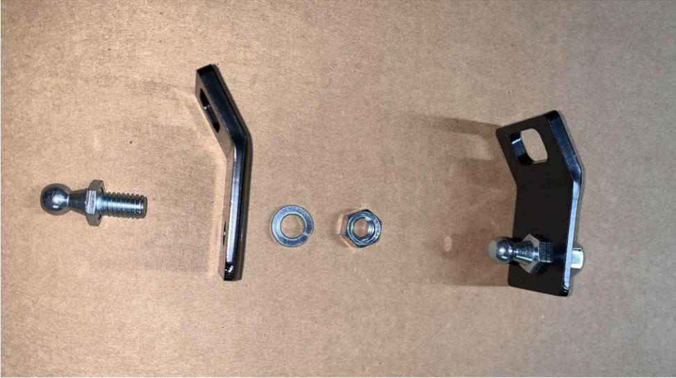
2. Remove the 1/2" bolt from your LH bonnet hinge channel, and replace it with the longer bolt (supplied), along with the flat washer and Bracket. Note that the bracket is made to be adjustable up and down the channel, but align it with the top end of the channel as shown. This photo shows the old design Flat Bracket, but installation is just the same with our improved Angled Bracket.
