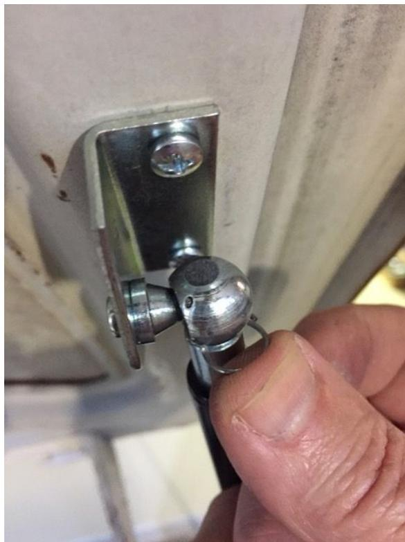
16. Periodically use a non petroleum-based lubricant on the struts and on your trunk gasket so their touching does not become abrasive. Dry Silicone Spray is ideal; available at ACE hardware stores.
