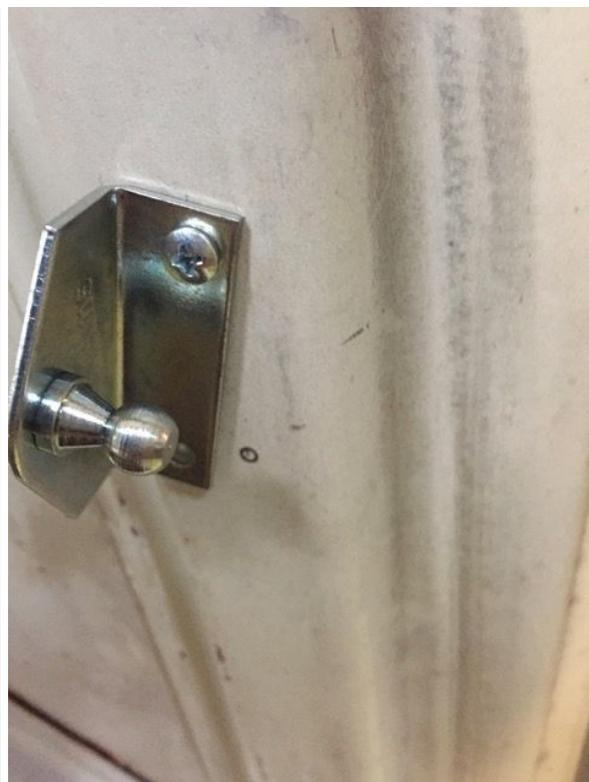
14. Attach the RH gas spring and test operation.
