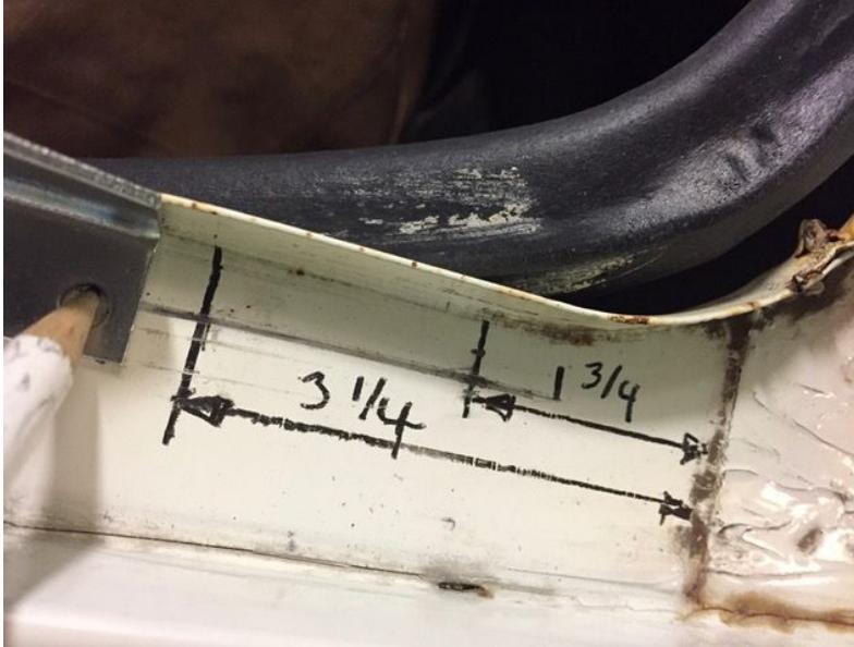
8. Center-punch the two points and drill with a 3/16" bit. Note: Use a tiny drill bit first if you like, to ensure accuracy. It is okay to drill a millimeter closer to the standing edge, but Not okay to drill any farther away, otherwise you will not clear your gasket upon final assembly.
