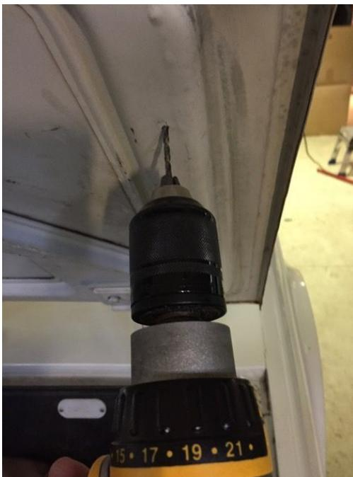
13. Remove the upper bracket from the strut and attach it to your boot lid with a sheet metal screw. A drop of thread lock is a good idea so the screw never vibrates loose. Now mark the second hole location, swing the bracket out of the way and drill the second hole. Fasten the second sheet metal screw (use a drop of thread lock) and tighten both.
