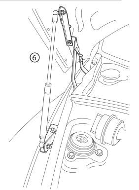
4. Attach a ball-stud along with lock-washer and nut to the right-hand lower bracket (see illustration below). Then install the bracket by removing the fender bolt shown, inserting the new bracket, and then replacing the bolt. Note: the bracket is positioned parallel to body line.
